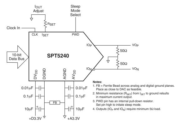
Figure 2: Typical Interface Circuit Diagram
